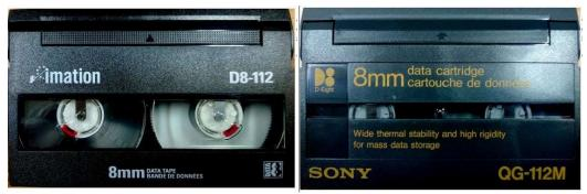
Fig 02: 8mm (Exabyte) tape cartridges
